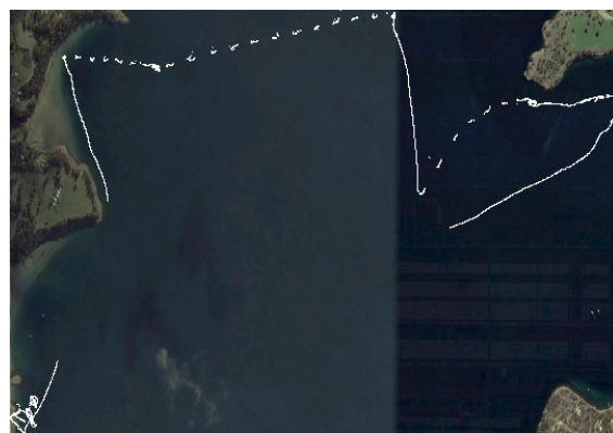
Figure 3. Typical Mission: AUV path traced in white from its mission start; bottom left, to end point; right center. The map shown covers an area of 3.76km horizontally and 1.84km vertically.
