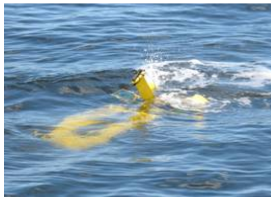
Figure 2. CSIRO's AUV 'Starbug' during the diving operation. The tail section is visible above water, which is approximately 0.5m in height.
