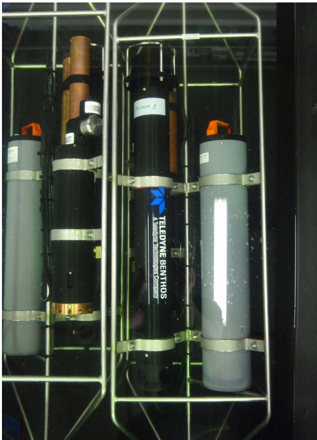
Figure 4. Sensor and acoustics packages mounted in frames for deployment at the NRS. The grey canisters are battery packs, the Teledyne benthos modems are labelled while the WQMs have copper components.
