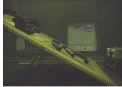
Figure 7. Tilt table with the blocks of logs in the water tank.
