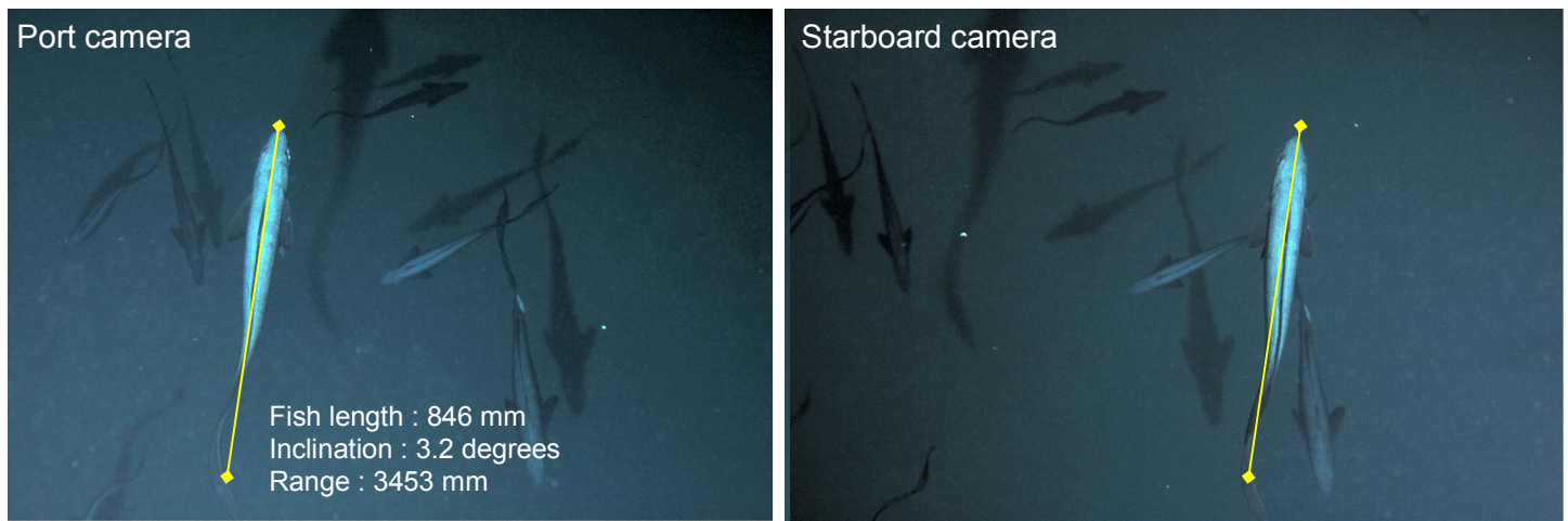
Figure 9. Blue Grenadier captured as a stereo image pair by the AOS digital stills subsystem showing example stereo photogrammetric derived metrics for one fish
