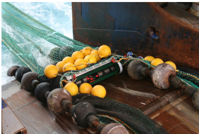
Figure 5. AOS attached to the trawl headline during deployment. Floats are attached to create a neutrally buoyant package when in the water.
