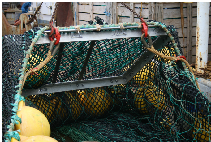
Figure 4. Mount frame secured to the headline of the trawl.
