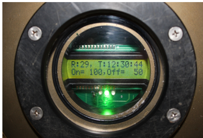
Figure 7. Acoustics module status display. Trigger depths for system activation are shown: power on below 100 metres, power off above 50 metres.
