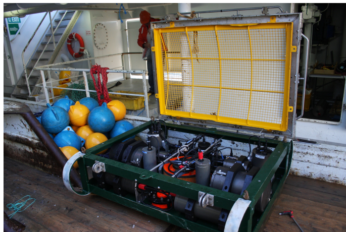
Figure 2. AOS System showing sled frame and hinged protective cover (yellow). Independent aluminium mount frame is shown bolted to the top of the protective cover.
