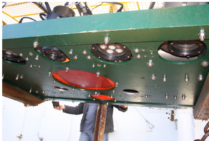
Figure 3. AOS underside showing Instrument Plate. Orange Simrad acoustic transducers are visible.
