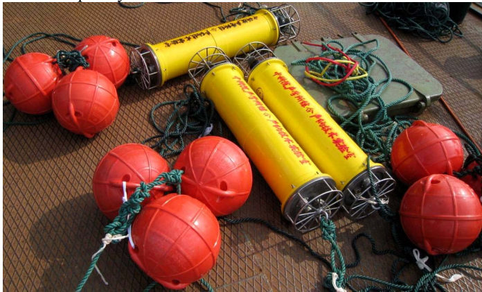
Fig.4 sensor network nodes equipped with SDA modem
