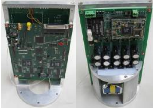
Fig.2 the compact electronic system of SDA modem: receive and processing module (left), transmit module (right).
