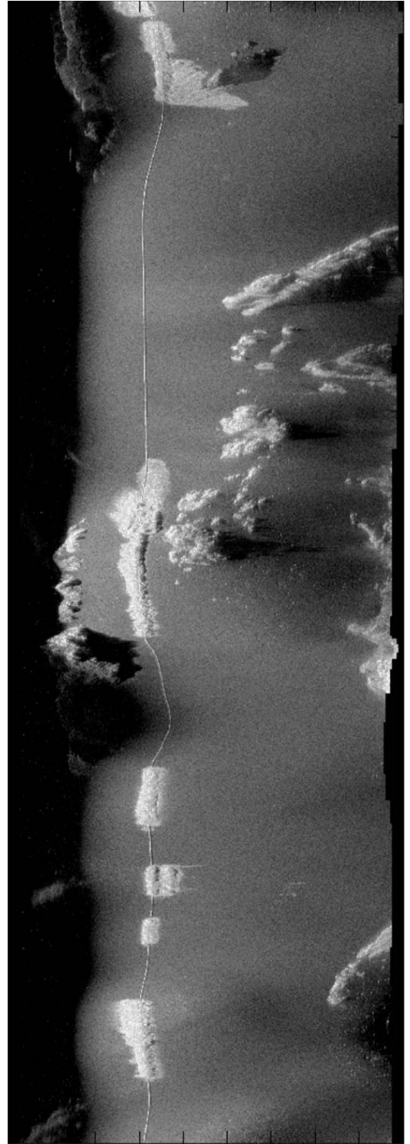
Fig. 6. Sidescan sonar image of the pipeline as a function of range and pings. The range is 0 m (left) to 180 m (right). The approximate distance travelled is 2000 m.
