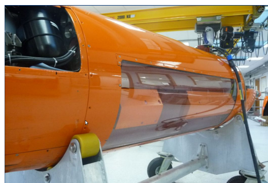
Fig. 2. The HISAS 1030 wideband interferometric SAS.
