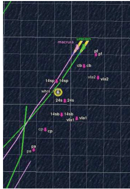
Fig. 5. The Google Earth interface for Ocean Vehicles (GEOV) [11] real-time topside situation display in Google Earth [12] showing two AUVs swimming in sync (trailed by purple and green lines) past an acoustic communications buoy (yellow circle) and a field of objects on the sea floor (pink arrows).
