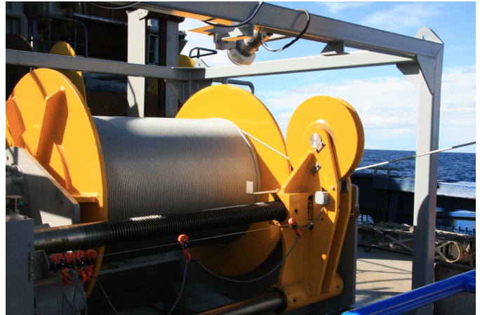
Figure 3. BOAGS winch with 6000 meters of cable
