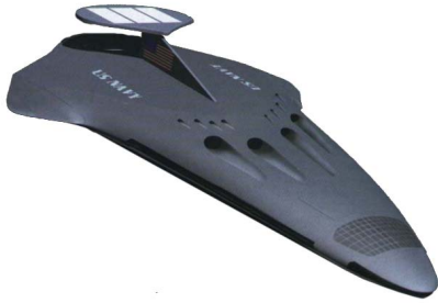
Fig. 2 Appearance of the NUWC's AUV Manta
