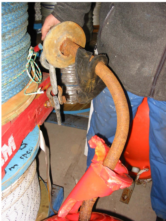
Fig. 4. Imploded 600mm plastic float.
