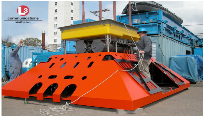
Fig. 17. The trawl resistant packaging for the node (Neptune Canada Photograph)
