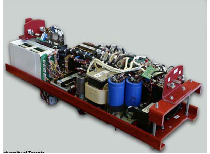
Fig. 10. The transmitter electronics. The package fits in a pressure vessel about 1 metre long
