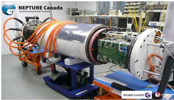
Fig. 16. The node electronics under testing at Alcatel (Neptune Canada Photograph)
