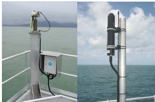
Figure 4. The CIMEL SeaPRISM (left) and the Satlantic HyperOCR (right) are mounted on the rooftop platform.
