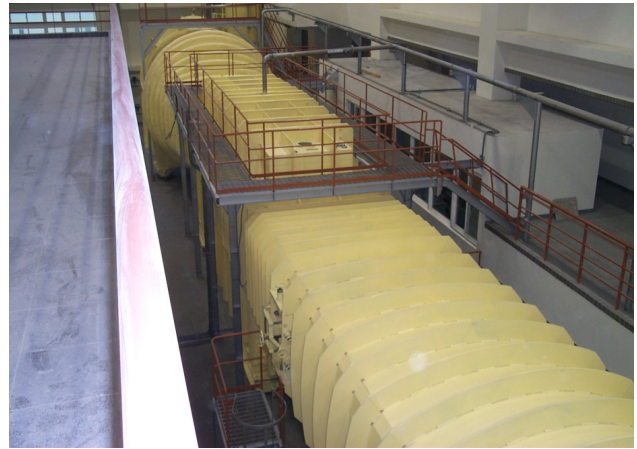
Fig. 8 The cavitation tunnel in the National Taiwan Ocean University.
