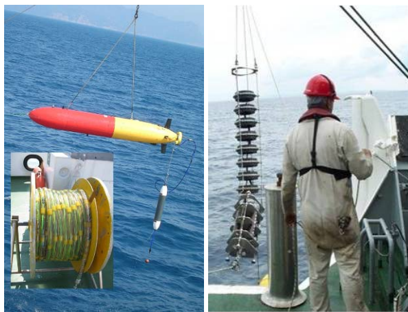
Figure 2. The photograph on the left shows one of NURC's autonomous underwater vehicles with its towed source (grey-white) which may also be used as a software defined modem transducer; in the bottom left corner the AUV's towed array can be seen on the winch. The photo on the right shows the moored sound source.
