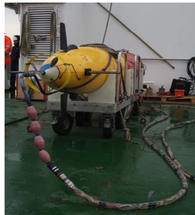
Figure 1. One of NURC's Ocean Explorer (OEX) Autonomous Underwater Vehicles (AUV) with a NURC towed array.
