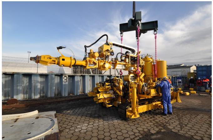
Fig. 1. Scaled multipurpose sub sea working unit of the project ISUP (founded by the German Ministry for Economics and Technology (BMWi), grant No. 03SX229A), courtesy of Aker WIRTH GmbH [7]
