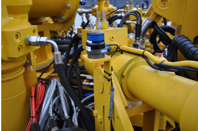
Fig. 2. One of the three responder units mounted onto the DWU, courtesy of Aker WIRTH GmbH
