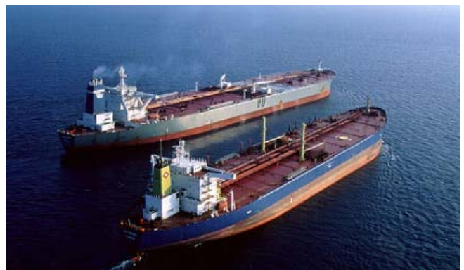
Figure 1. Lightering Operation[3]: The two vessels have come alongside and commenced mooring operation while still underway at slow forward speed.
