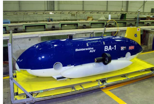
Fig. 1 Target hovering AUV of this study, which has been developed by the research group at Tokyo University of Marine Science and Technology, Japan. The AUV has four horizontal thrusters for surge, sway, and yaw motions and two vertical thrusters for heave and pitch motions.
