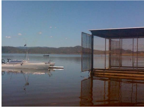
Fig. 11. The ASV can undertake more complex tasks requested remotely via the sensor network such as “dock into the security cage”.
