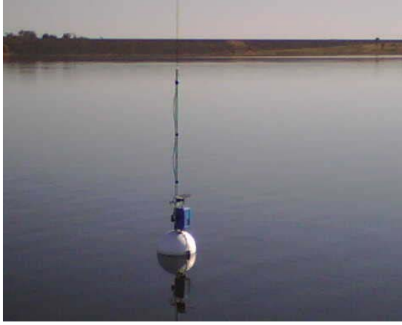
Fig. 6. A floating lake sensor node as used in the evaluation trials.
