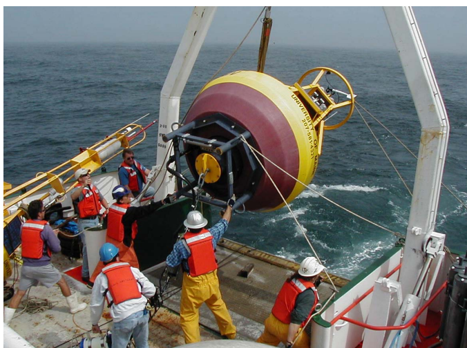
Figure 3. University of Maine oceanographers deploying a real-time data buoy from the RV Cape Hatteras.
