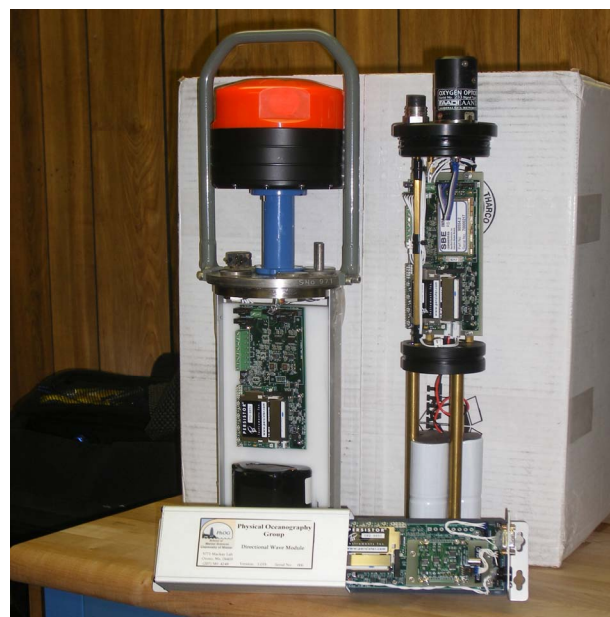
Figure 4. The serial bridge as the electronics and data logger of an Aanderaa z-pulse current meter sensor, as a data logger and inductive modem for the Aanderaa Optode, and as part of a directional wave sensor to be mounted within the buoy electronics well.
