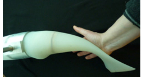
Fig. 6. The lateral buckling problem for the tail made of Dragon Skin A10 with hollow mid-section.
