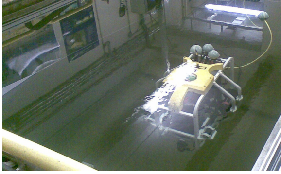
Fig. 5. The autonomous underwater vehicle Nessie IV in the OSL tank. It is to be noted the division panel, in order to create two identical environment sections.
