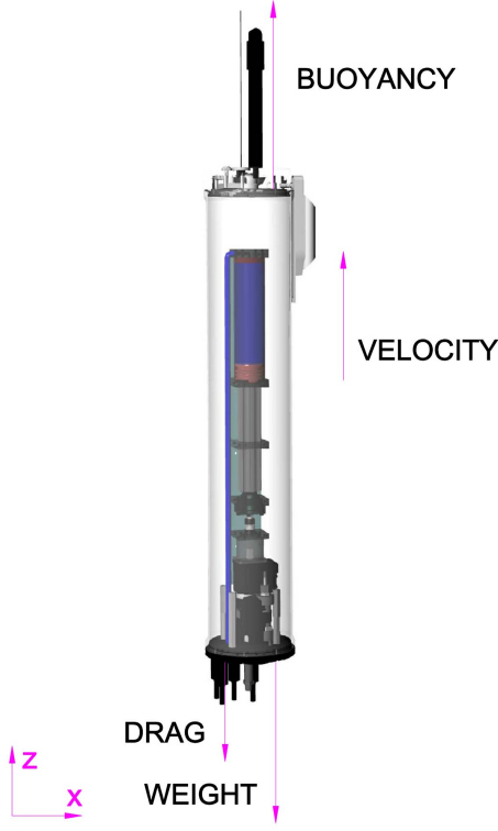
Fig. 4. The main forces acting on the moving float. The float is assumed to be ascending and therefore the buoyant force is greater than the weight of the float. As the float moves, it is also subject to a quadratic drag force. Additionally, an added mass term is considered, which accounts for the additional inertia provided by parcels of water working against the accelerating float.
