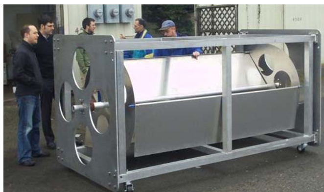
Figure 2. A displacement-type Flip Wing hydrokinetic turbine for electricity generation at low water velocities. Photo courtesy of Hydrovolts Inc.
