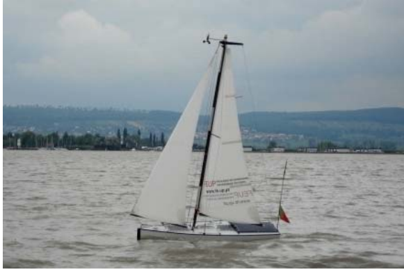
Fig. 1. FASt – the FEUP Autonomous Sailboat.
