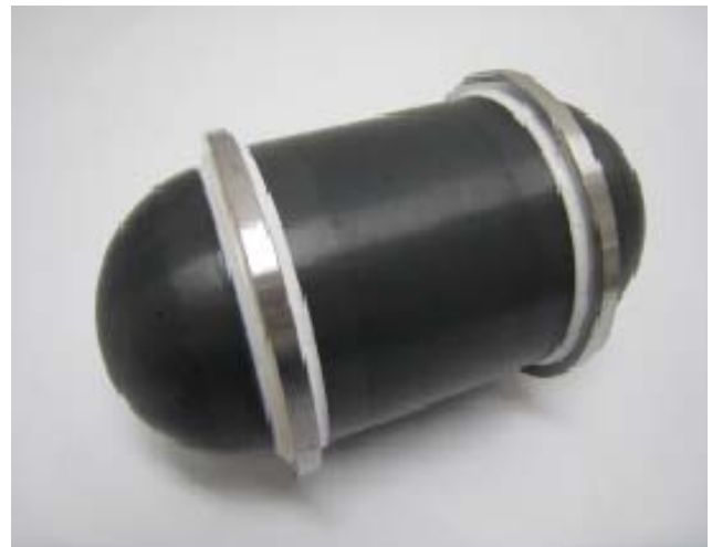
Figure 2 Photo of the small model for ceramic pressure housing which can withstand 120 MPa hydraulic pressure.
