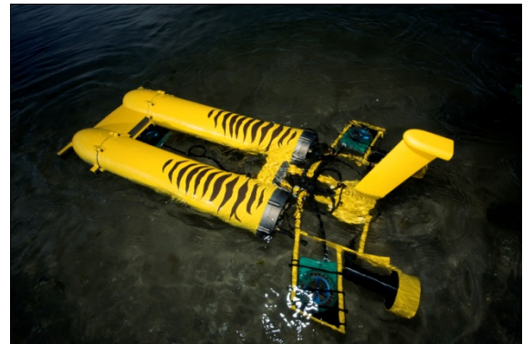
Figure 1. The Autonomous Underwater Vehicle (AUV) developed at CSIRO. This AUV is 1.2-m long and is equipped with different sensors.
