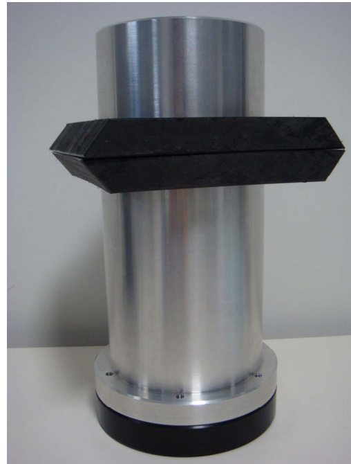
Figure 3. Housing for X-ray spectrometer to allow it to be attached to an AUV. Dimensions are 28 cm long, 11 cm in diameter. The X-ray tube and the radiation detector are placed in the vertical position (pointing down).
