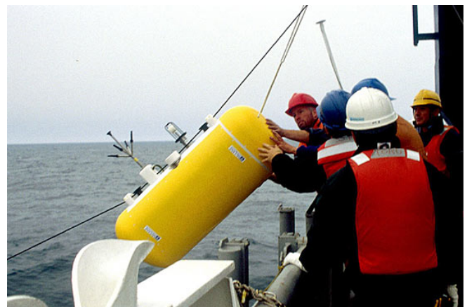
Fig. 1. McLane Moored Profiler being deployed.
