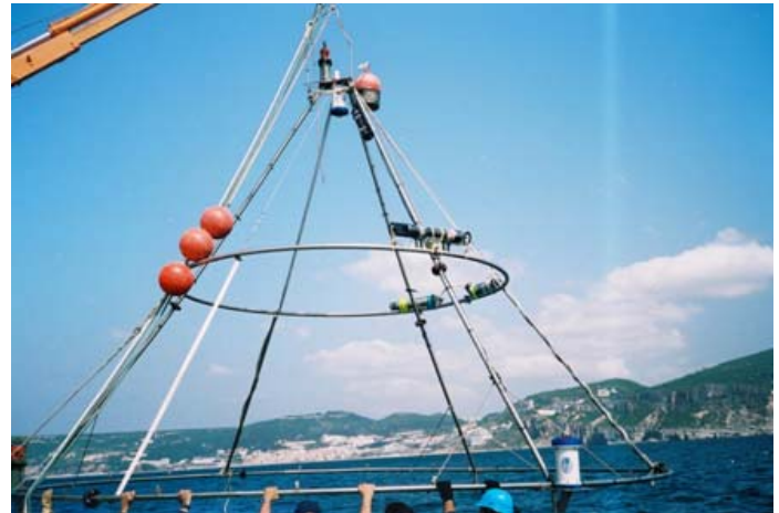
Figure 6. The CORSED platform being deployed during a test, showing the two ADCPs, the two RCM-9 and the LISST.
