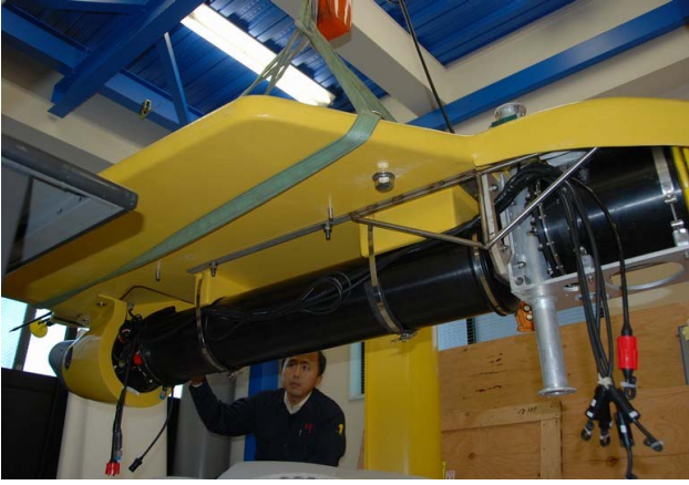
Figure 2. Assembly of the surface platform based on a S-AUV. The S-AUV system and the sea surface unit including acoustic ranging system, GPS receiver, motion sensor were installed into two cylinders for installation onto the S-AUV.
