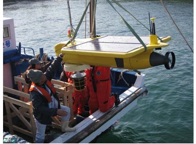
Figure 3. Deployment of the S-AUV-based surface platform using the davit equipped on the small working ship.
