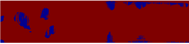
Fig. 10. Difference bathymetry after applying threshold, red - flat areas; blue - bumpy areas
