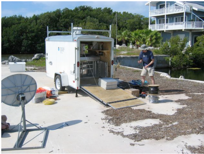
Figure 3. Mobile SeaSonde developed by NOAA CO-OPS being deployed in Key Largo, FL, USA.
