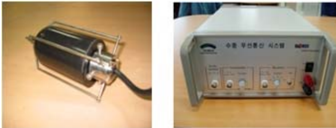
Figure 1. Photos of implemented omni-directional acoustic sensor(left) and transmitting and receiving amplifier to derive omni-directional sensor (right)
