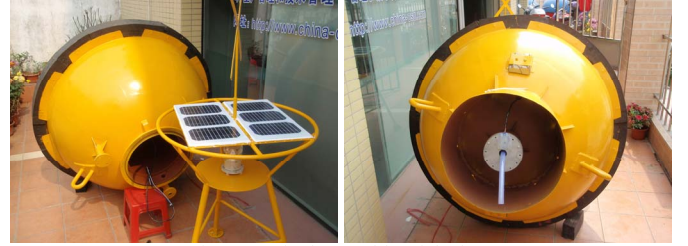
Figure 6. Final assembly of the buoy
