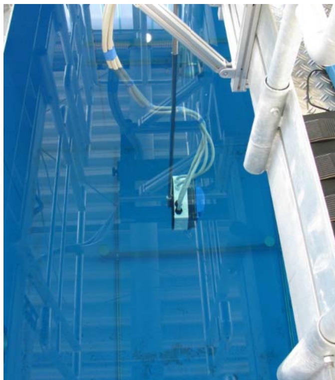
Figure 13. System qualification in measurement tank 6m x 8m x 6m for farfield measurements
