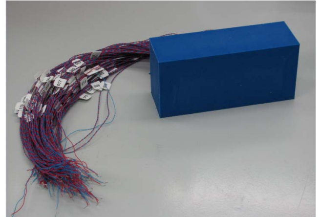
Figure 10. Image of a receiver test antenna for performance assessment
