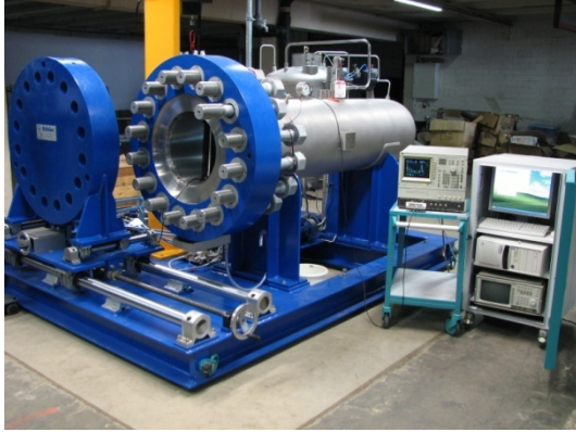
Figure 6. Pressure chamber (diameter 440 mm, volume 385 ltr.) together with external measurement equipment.
