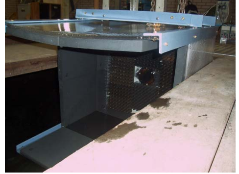
Figure 5. Transducer encased in acoustic absorbing material.
