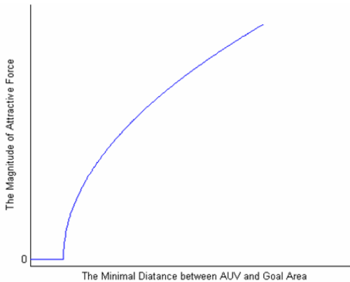
Figure 2. The component of the attractive force versus the minimal distance between AUV and the goal area.
