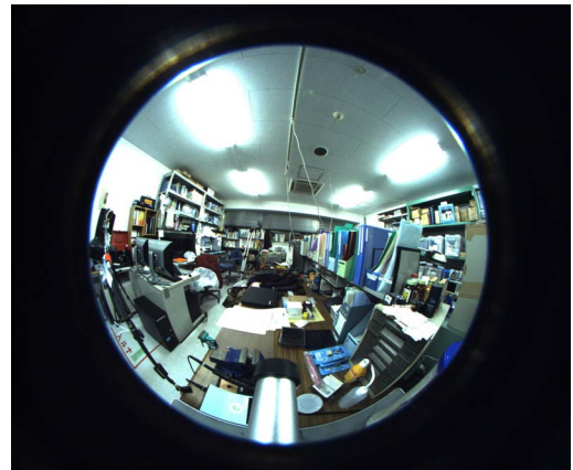
Figure 4. Raw image taken by the prototype of the low distortion all-around view system.
