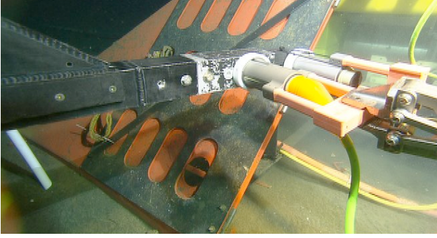
Fig. 5. MBARI ROV Ventana preparing to plug in the power and Ethernet cable from the modem node.
