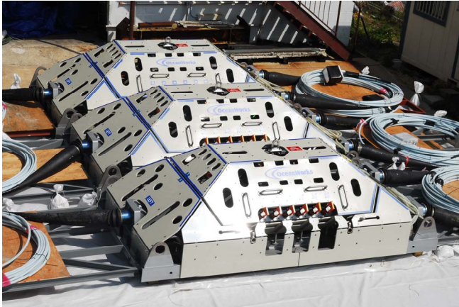
Figure 4. Seafloor nodes being readied for deployment
