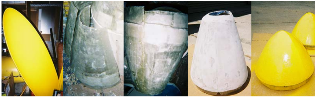
Figure 3.8 (a-e) Process used to create end caps from left to right: a) existing AUV shell used as a mold, b) end caps were created in halves, c) halves were joined, d) end caps were sanded and filled, and e) end caps were painted
