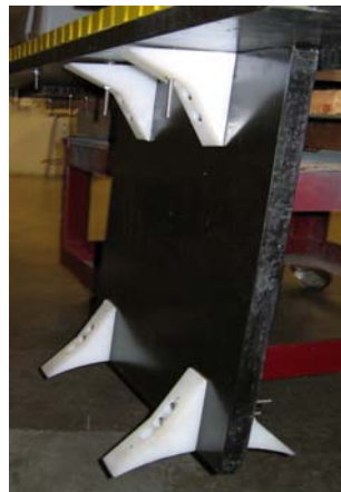
Figure 3.30 UHMW clamps fastened to vertical struts
