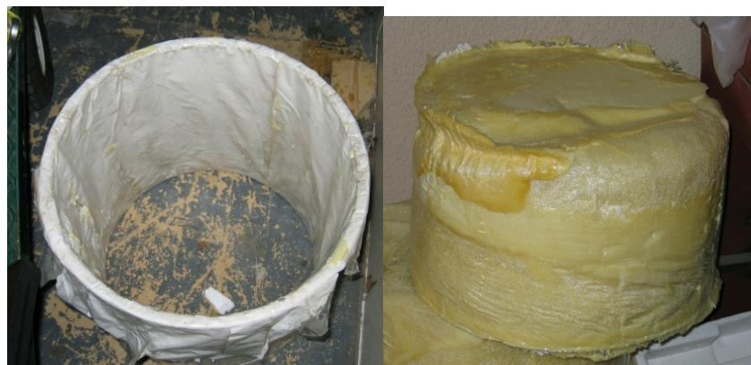
Figure 3.9 (a,b) a) Picture of the Mold for the Foam and b) a Foam Insert
