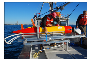
Engineers Hoover (left) and Hobson (right) prepare to deploy the Long Range AUV on the Launch and Recovery System (LARS) designed at MBARI.
