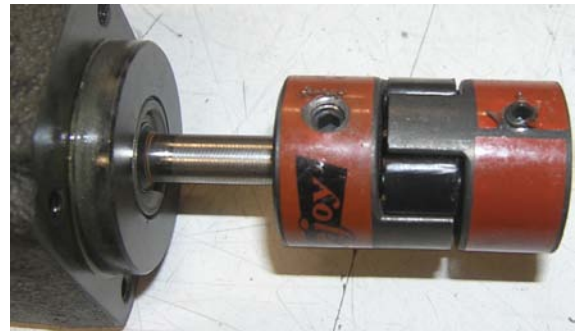
Flexible coupling on pump shaft
