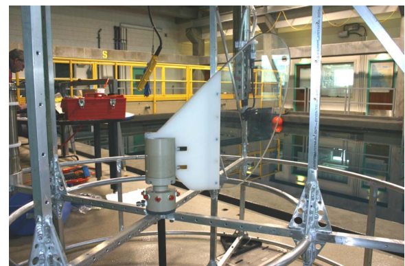
Fig. 4: Directional Valve Assembly in FOCE Frame
