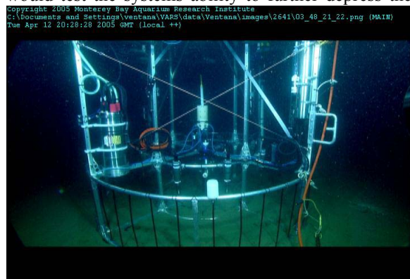
Fig. 10: FOCE deployed in the Monterey Bay
