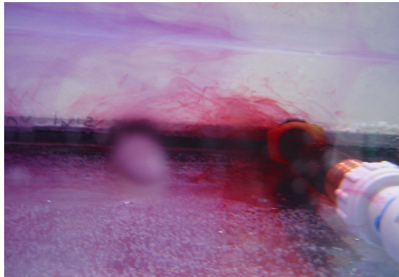
Fig. 5: Soaker hose was selected for HCl release after testing a variety of methods
