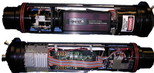
Fig. 4. The integrated camera, lens, VLIC and supporting electronics in their housing mounting bracket.
