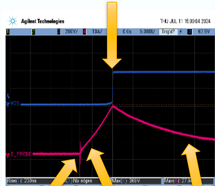
MOSFET TURNING OFF (200ns)
