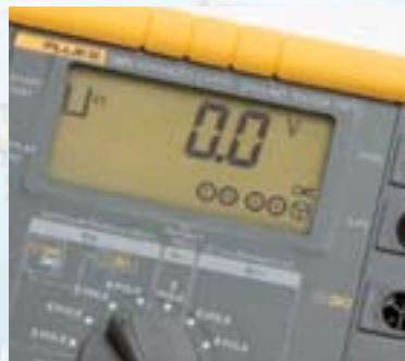
Use the Fluke 1625 to determine the health of your earth ground systems.
