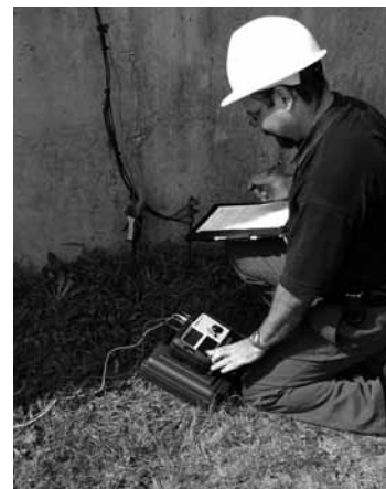
Using ART method with Megger DET3TC to test commercial ground without disconnecting the system
