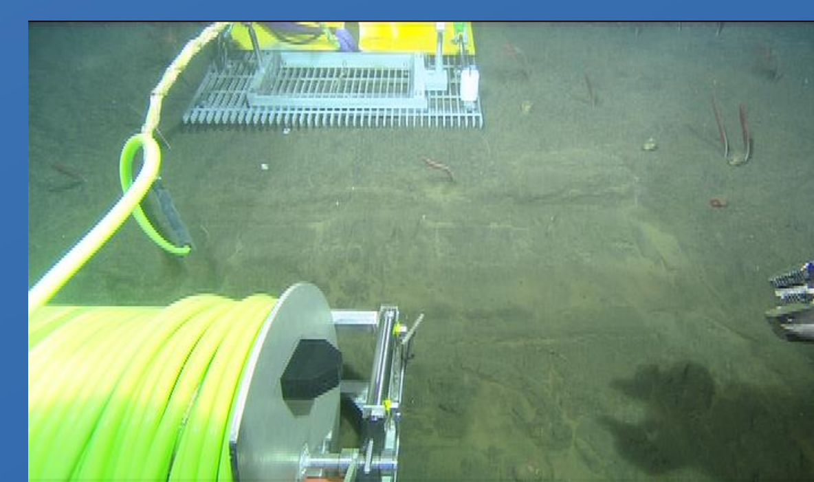
Deploying the cable to the MARS node
