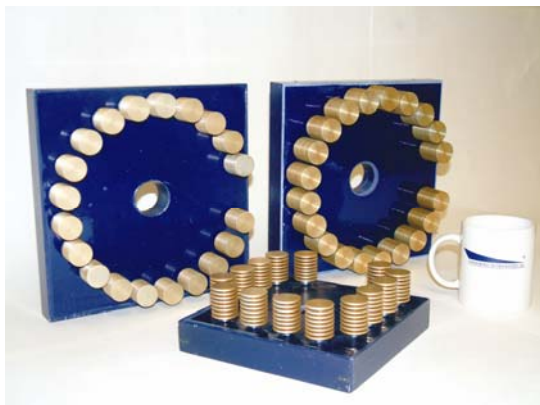
Figure 4. PowerMod™ high-voltage solid-state switch modules. The larger switches consist of 20 IGBTs in series and are rated for 10 kVDC at 100 A peak current.
